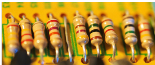
Resistors wired into a computer circuit board. Each resistor has a color code that indicates its resistance in ohms.
